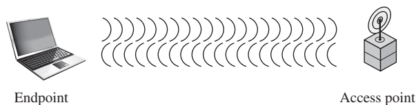
Figure 24.1 Wireless Networking Components
